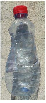
Figure 5: Plastic bottle crushed by change in atmospheric pressure when it was filled with air at a high elevation and carried to a lower elevation. (Source: David Monniaux)
